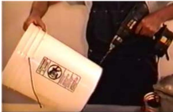
Uncoil a short length of the copper coil to stick out of the hole at the bottom of the Cooling Bucket and place the coil inside the Cooling Bucket.
